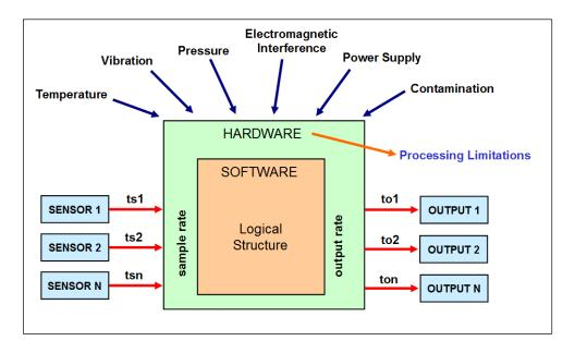
Figure 4 – Simplified schematics for hardware and software interface.
