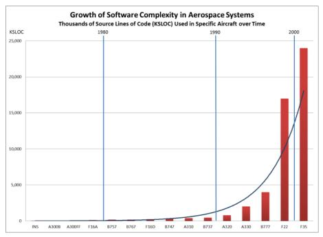
Figure 1: Growing of software complexity in aerospace systems [13]
