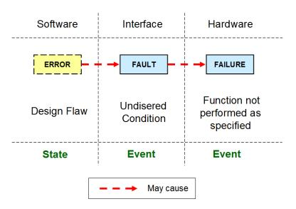
Figure 2 – Representation of error, fault and failure.
