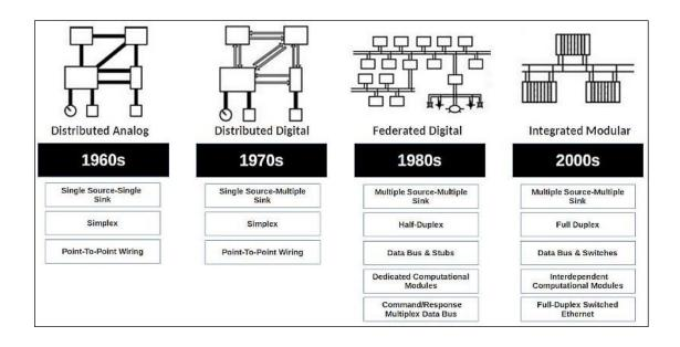
Figure 3: Growing level of integration in avionics architectures [8].
